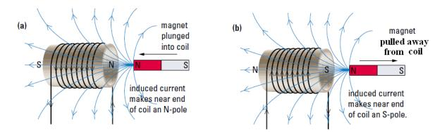
Lenz's Law is really an application of the Law of Conservation of Energy. It wouldn't make sense that, when you induce a current by moving a magnet, the new magnet field created by the current would "assits" the initial motion.
