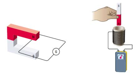
Key to his discovery was that **you needed to move the magnetic field** relative to the wire to generate current. If the wire was exposed to a **changing** magnetic field, current would flow through it.
