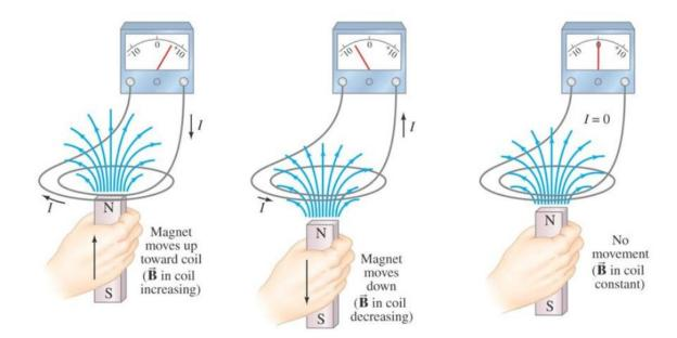
By observing what happens when a bar magnet is plunged into the core of a coil that is connected to a voltmeter, it is possible to conclude that the factors affecting the magnitude of the induced current are:
